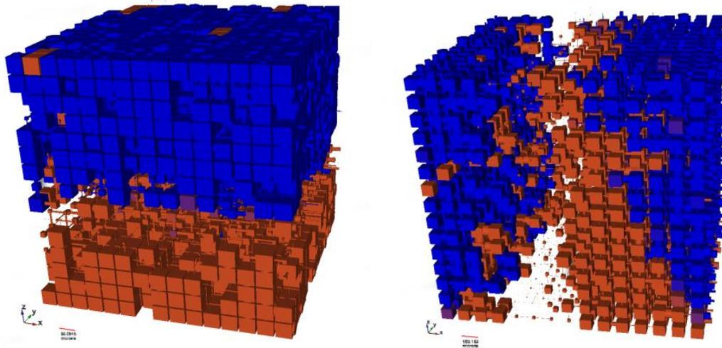
Figure 4A & 4B – Where 4A shows the wetting simulation after 10 ms for sample A. The wetting fluid is shown blue. 4B demonstrates the wetting simulation after 10 ms for sample B.
