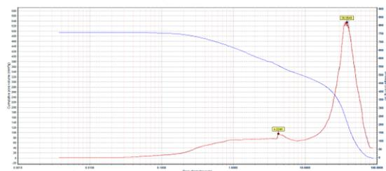
Figure 1- Mercury intrusion porosimetry curve (blue) and its first derivative (red) for sample A.
